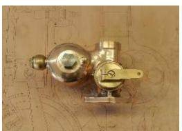
Solex Bronze Body Barrel Throttle Carburettor
